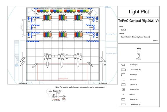
The TAPAC lighting rig consists of a 6 zone front light of 1.2K Fresnels, with a similarly split RGBA top light setup. There are 3 generic specials above audience, and 4 more high side specials from the balcony area. Any reasonable changes that wish to be made to the lighting rig within the allocated hire time can be done with no extra charge. (This includes resetting the rig).
